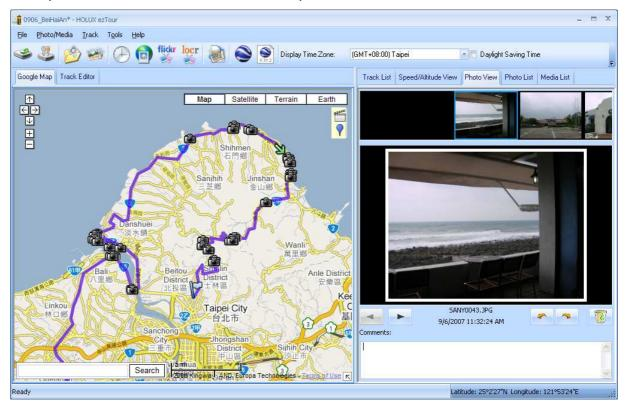
When photos are added, GPS Photo Tagger will automatically match photo and GPS logged waypoints by time. Place marks will be created as a placeholder for photos.
